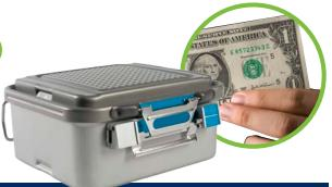
**Objective**: To determine if there is a breach in barrier protection for rigid sterilization containers. To maintain sterility, after terminal sterilization has been attained, rigid sterilization containers should provide a complete seal between the lid and the container case. If not, the seal is compromised and hence a breach in barrier protection has occurred.
